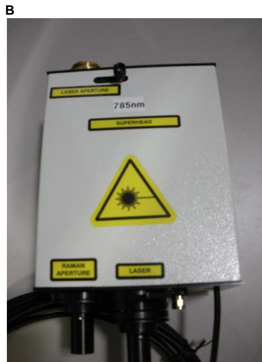
Photo 5: Raman probe head. (A) full view positioned for collection, (B) full view free, (C) bottom front, (D) base of probe head with fiber optic input port (center) and Raman collection port (left)
