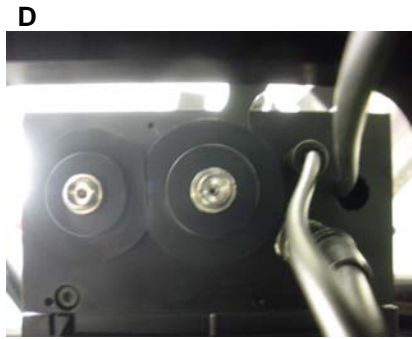
Photo 6: View of the laser focusing lens in line with the goniometer (blue arrow). Note: the configuration shown is for absorption collection. For Raman collection, the probe head lens is positioned using remote control to be in line with the crystal.
